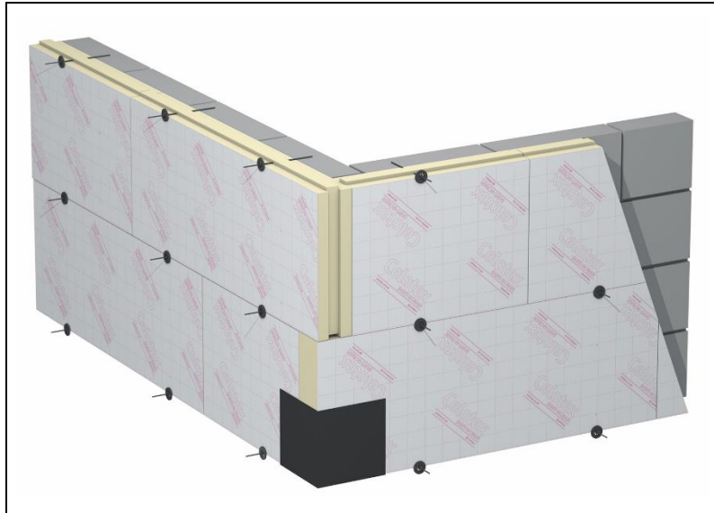
Figure 5 Corner board blocking arrangement
