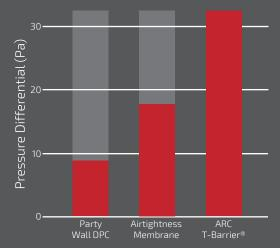
lesults presented were obtained using a 100mm party wall avity with a 100mm external cavity.
