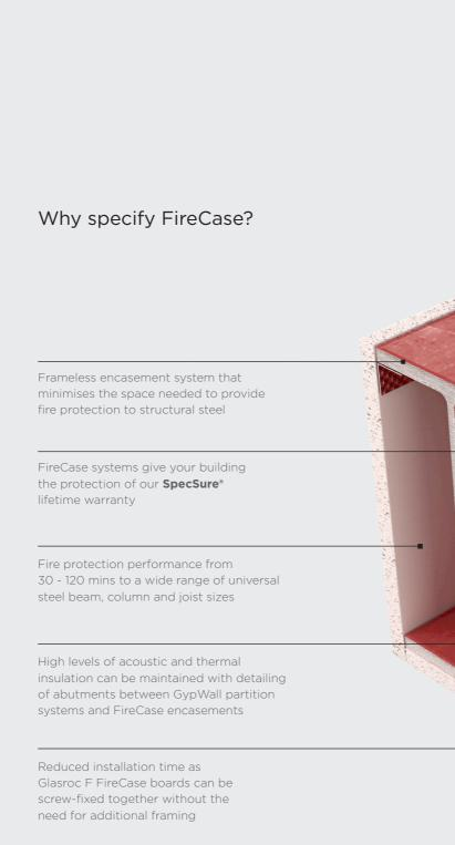
Build-programme flexibility and earlier installation as the inherent moisture resistance capability of Glasroc F FireCase means that installation of the FireCase system can begin before the building envelope is fully weathertight. Only suitable for temporary exposure such as during installation
