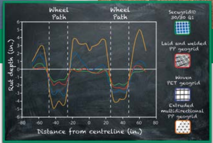
Fig. 22 Comparison of rut depth at 300 truck passes, Montana field trial (Phase 2, 2014)
