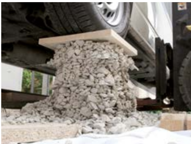
Fig. 5 Interlocking effect of Secugrid®/Combigrid®. Radial movements on the base course causes a torsional momentum in the junctions
