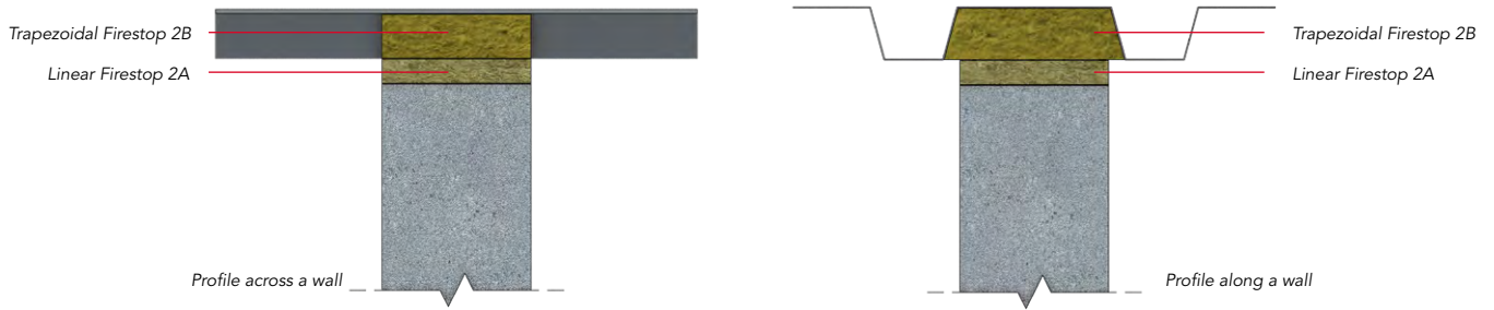
Figure 4 Profiled metal deck over blockwork wall
