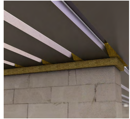
Figure 3 Linear Firestop 2A and Dovetail Infill Strip
