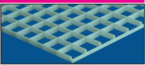
The TS Premium opal eggcrate louvre is designed to be a rigid product with a good visual cut off. This louvre has a cell configuration of 15 x 15 x 13 mm. It is injection moulded on the most modern computer controlled system and each individual louvre is coated with an anti-static fluid to prevent the airborne dirt and dust from sticking to the cell walls during installation.
