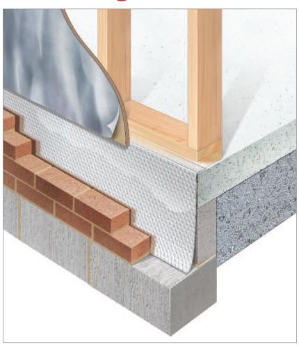
A simple and low cost solution for insulating the edges of ground floor slabs to prevent cold bridging.
