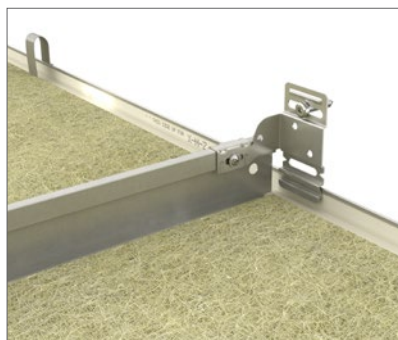
To ensure the squareness of the Rockfon System T24 X it is recommended to use a wall bracket on every main runner and every second cross tee.
